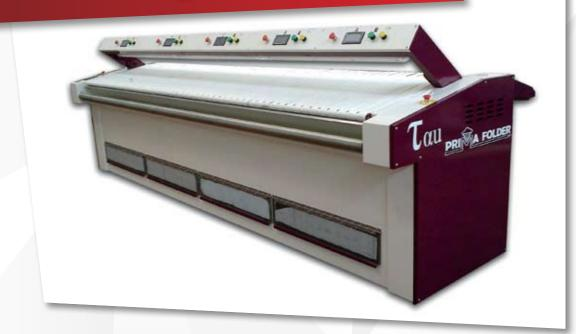
**TAU** is a machine designed to facilitate and speed up the operation manual of feeding of flat linen of various kinds; from small items such as towels and pillowcases, to medium and large items as tablecloths, tablecloths guards and bed sheets.
