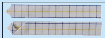
三尖側貼 (底斜角) Bottom inclined triangular sleeve placket
