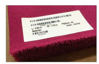
When the spread is complete, the spreading system's wireless barcode printer generates a barcode label to attach to the top ply of the spread. The spread then travels to the Paragon® cutter. The cutter operator scans the barcode to retrieve the proper cut file.
