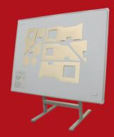
Place existing templates on the digitizer surface and capture perimeter and internal geometry
