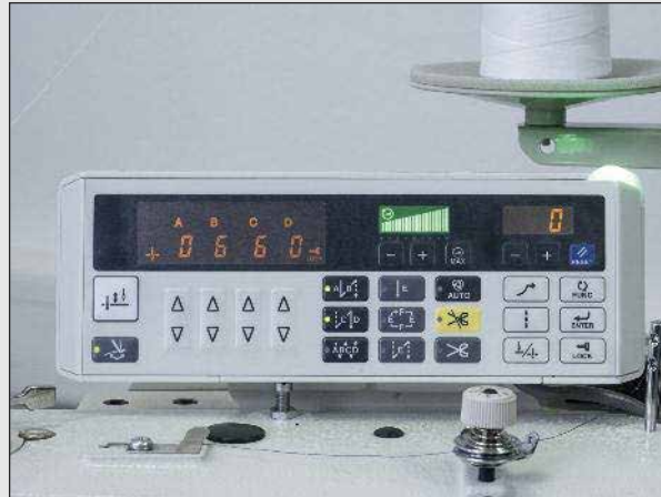
Control panel for adjusting various sewing functions
