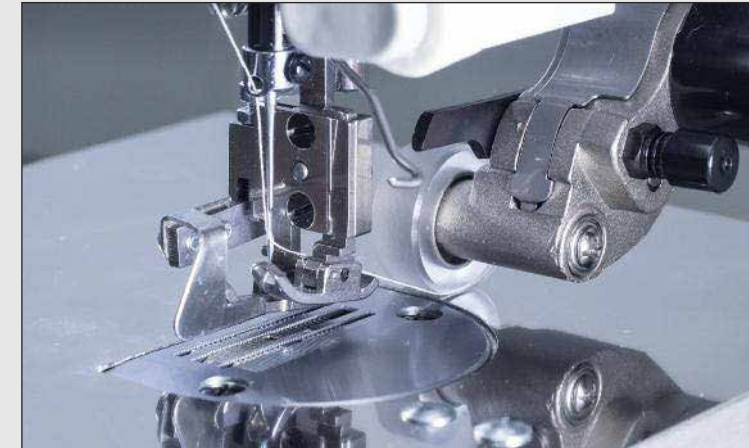
Special presser foot for stitching in the shadow of the seam
