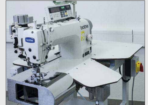
Working table shaped for ease of production
