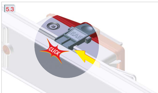
Be sure that, the box is fixed to the busbar properly.
